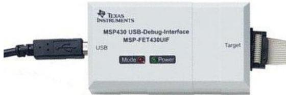
This application note contains hints for using the MSP-FET430UIF interface together with a Merifix test fixture, to make a self-contained programming fixture suitable for use in the engineering lab or in low-volume production.
