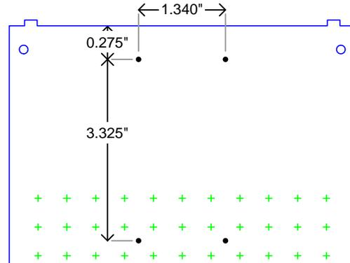
The original screws are about 0.7" (18mm) long. Suggested longer screws are #4 x 1" self-tapping Philips pan head. The holes in the probe plate can be 1/8" (3.2mm) for clearance.
