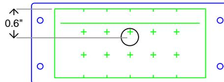
You only need the hole to be big enough for the metal part of the USB plug. The rear insert is thin enough that the moulded plastic part of the plug does not need to pass through it.
