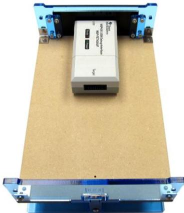
Mounted like this it encroaches about 1" into the centre of the probable area. The photo shows one mounted below the probe plate of an MF500 fixture. On the MF300 fixture there is a little less room, but there is enough space for probes at the front if the DUT is small.
