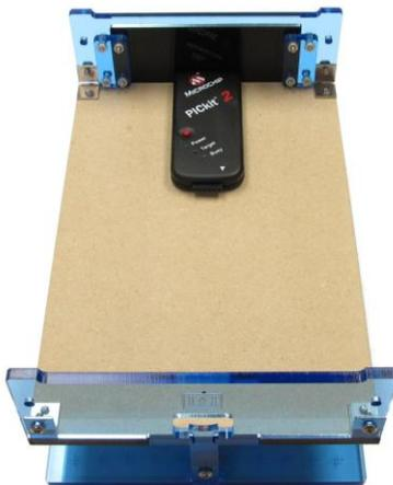
The small "lanyard" loop on the end of the enclosure must be trimmed off so the USB connector can be flush with the rear panel insert. A sharp knife removes it easily.
