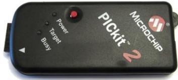
This application note contains hints for using the PICKit 2 or PICKit 3 interface together with a Merifix test fixture, to make a self-contained programming fixture suitable for use in the engineering lab or in low-volume production.
