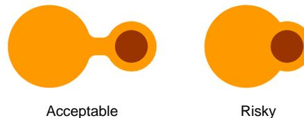
This creates the danger of test probes slipping into the via hole and being bent off-centre, which will reduce pointing accuracy and can cause probes to jam.
