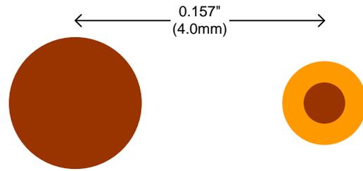
If there are limited places on the top side of the board where hold-down posts can land (areas free of components), avoid placing test points on the bottom side directly under those locations. On the fixture you don't want hold-down posts directly opposite test probes, because the hold-down posts can hit the test probes if the fixture is closed with no board in place.
