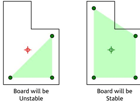
Keeping the largest possible distance between the holes maximises alignment accuracy.
