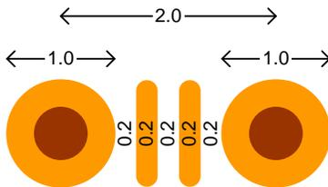
If routing density between test points is not crucial the pads may be made a little larger if desired. This relaxes the pointing accuracy required of the test probes and can make for a more reliable fixture. Pads can be enlarged up to 0.056" or 1.4mm and still leave space to get a single trace between adjacent test points.
