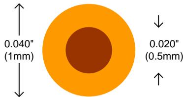
The hole can be a little smaller than suggested if desired - perhaps to make it the same size as via holes on the board. But don't make it too small. The smaller it is the less effective it will be at helping slightly misaligned probes to self-centre.
