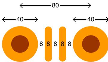
Similarly, 1mm test points on a 2mm grid allows two traces between test points using common 0.2mm trace/space rules, routing on a 0.1mm or 0.2mm grid.
