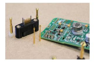
Check the mechanical operation and alignment. At this stage the Tag-Connect probe is just pressed in to the Tag-Mount so it may move down as the fixture is closed, but it will be possible to check the positioning, orientation and smooth operation.
