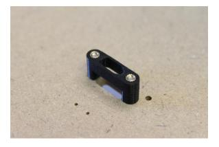
Fit the Tag-Connect probe from the underside of the probe plate. The hole in the probe plate is a clearance fit and the opening in the Tag-Mount is a snug slip fit.
