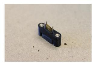
Fit the remaining test and locating probes to the probe plate in the normal way.
